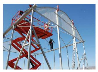
the acceleration and fall force experienced by an approved fall arrest test dummy, fitted with sensors in the critical impact areas (cranial and lumbar zones) and dropped from different parts of the greenhouse roof (including ridge and gutter). The validation of the system has been carried out at the Tecnova Experimental Centre, thanks to the financing provided by the Andalusian Institute for HSE (part of the Ministry of Employment, Business and Trade within the Andalusian Regional Government).
